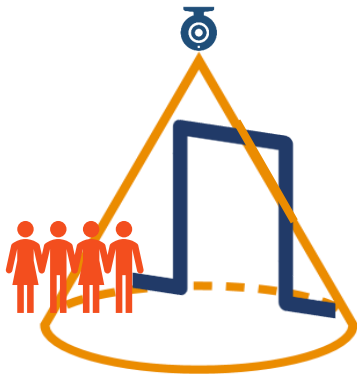
Illustration 13: Side view of a door and the optimal coverage radius of a camera
