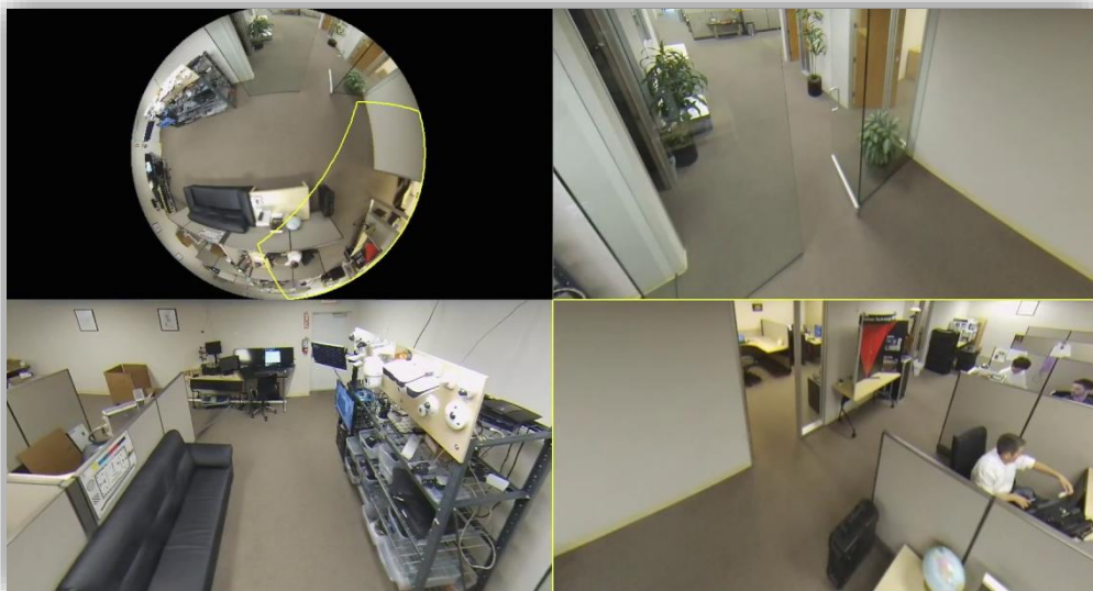
Illustration 12: Top left: Original image of a ceiling-mounted fisheye camera. All others: Images "dewrapped" from the original image
